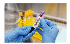
On top of this, the B-492 'FreezerBondz' label that could now be printed almost automatically, with the BradyPrinter i3300 isn't just any label. It perfectly fits tubes, can resist common laboratory chemicals, and the label stays legible and attached under liquid nitrogen storage temperatures at -196°C.
