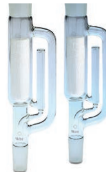
Fig 13. Extraction thimbles in Soxhlet extraction apparatus.
